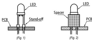
3. Use stand-offs (Fig.1) or spacers (Fig.2) to securely position the LED above the PCB.
