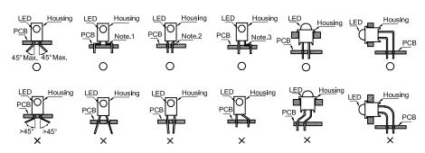
O" Correct mounting method " x " Incorrect mounting method
