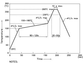
We recommend the reflow temperature 245°C(+/-5°C).The maximum soldering temperature should be limited to 260°C.
